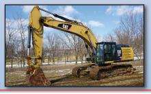
**2013 CAT 320E LRR**, s/n TFX00662, Cat C6.6 diesel and hydraulic drive, 9'6" dipper stick, Cat 24" digging bucket, Cat hydraulic coupler, aux hydraulics, pattern changer, rearview camera. EROPS with heat and ac, and 31" TBG pads with bolt-on street pads. In good condition with good undercarriage. (7,017 Hours) (EX-207) (Derry Lane -Blairsville) (Purchased New)
