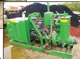
(1) of (2) 8" x 6" Diesel Pumps
