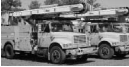
(2) ALTEC LBM500C, 50' Matl. Handling Aerial Lifts
