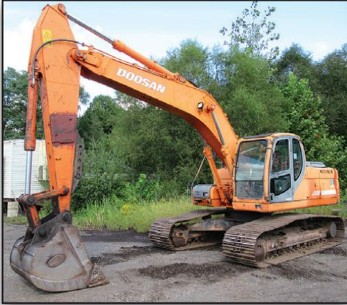
**DOOSAN Model DX225LC Hydraulic Excavator**, s/n 70005038, powered by Doosan diesel engine, equipped with 9'6" dipper stick, Geith 42" digging bucket, thumb bracket, pattern changer, enclosed ROPS cab, and 31.5" TBG pads. In fair to good condition with fair to good undercarriage.
