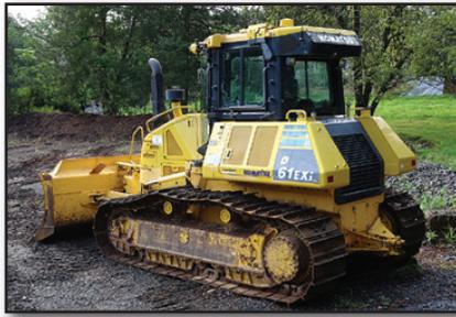
**2017 KOMATSU Model D61EXI-24 Crawler Tractor**, s/n B60119, powered by Komatsu SAA6D107E-3-A diesel engine and hydrostatic transmission, equipped with 6-way straight blade, Intelligent Machine Control integrated GPS, rearview camera, drawbar, and 24" SBG pads. In good condition with good undercarriage. **(Purchased New)**
