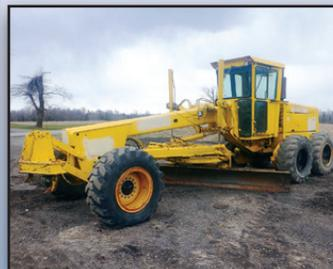
**JOHN DEERE Model 770B Articulated Motor Grader**, s/n 77006491T, powered by JD diesel engine and 8 speed powershift transmission, equipped with 12' fully hydraulic moldboard, front scarifier, enclosed ROPS cab with heat, and 17.5x25 tires. In good condition with good tires.
