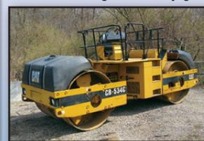
**1998 CATERPILLAR Model CB-534C Tandem Vibratory Roller**, s/n 5HN00326, powered by Cat 3054 diesel engine and hydrostatic transmission, equipped with 65" smooth drums, front and rear spray, and vibrating drum selector. In good condition. (Meter Reads 04,675 Hours)
