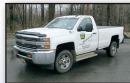
**2015 CHEVROLET Model 3500HD Crew Cab Utility Truck**, powered by Duramax 6.6L Turbo diesel engine and Allison automatic transmission, equipped with Reading 9' open utility body with topside box and material rack, dual rear wheels, tow package with electric, cruise control, power windows, locks, and mirrors, air conditioning, and 235/0R17 tires. In good condition with good tires. (Odometer Reads 205,275 Miles)
