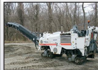
**2001 WIRTGEN Model W1200F Milling Machine**, s/n 07-10-110123020221, powered by Deutz diesel engine and hydraulic drive, equipped with 48" milling head, spare 36" milling drum, 24" hydraulic discharge conveyor, and (4) independent crawlers with bolt-on poly street pads. In good condition with good undercarriage. (Meter Reads 2,856 Hours)
