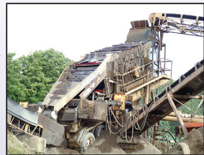
HYDRAULIC WASH PLANT
